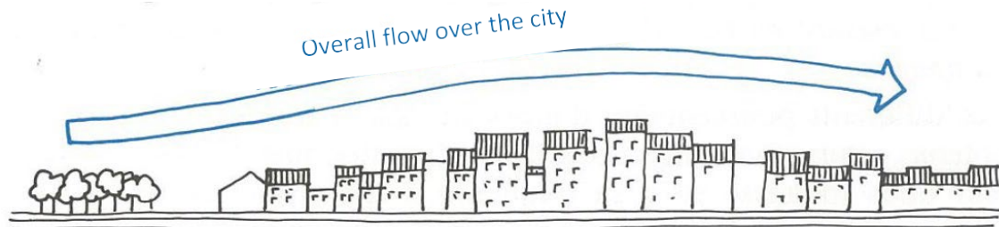
Figure 10: The wind does not penetrate into densely packed buildings
