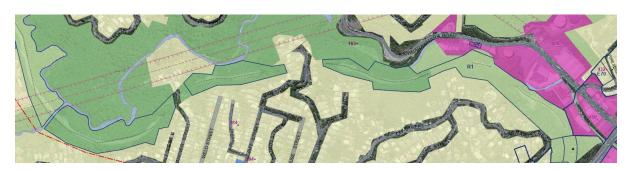
Snip from the Operative Wellington City District Plan 2000 eplan in relation to Tunnels 1-5 on the Johnsonville line which shows breaks in the mapped designation. The designation has references of R1-R5. All of the KiwiRail tunnels were mapped in this manner.
