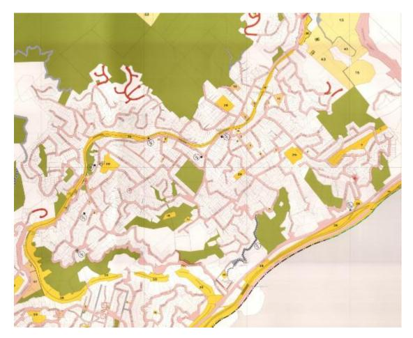
Snip from the Operative Wellington City District Plan 1985 in relation to Tunnels 1-6 on the Johnsonville line which shows breaks in the mapped designation over the tunnels. The designation reference in this plan was '38'. All of the KiwiRail tunnels were mapped in this manner.
