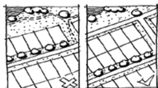
Poor lot orientation shown at left with backs of lots connecting to the park. Preferred orientation with
