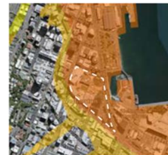
Figure 16: Liquefaction potential (source: WCC)
