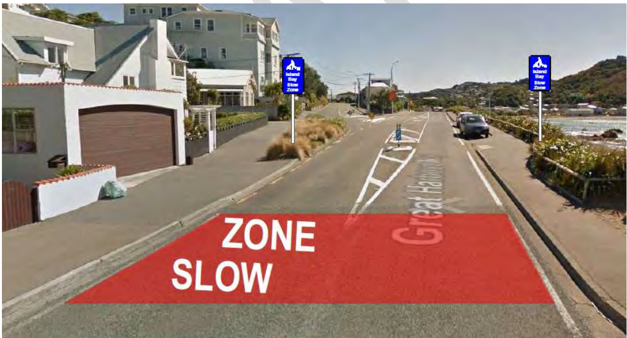
Figure 10: Island Bay example of a 'Slow Zone' - road marking and signage
