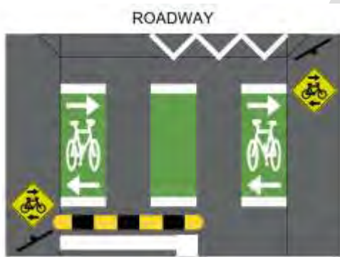
Figure 15: Recommended bike path treatment across driveways
