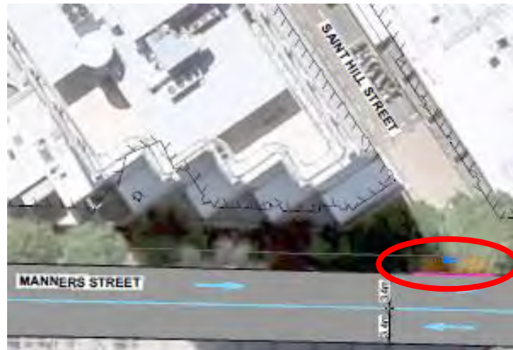
Figure 19: Footpath widening at location of sump on Manners Street
