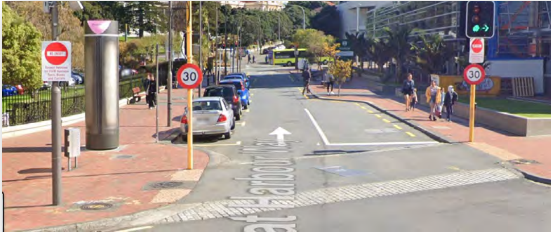
Figure 6. An Example of Side Street Access Control - Bunny Street, Pipitea (Google Streetview)
