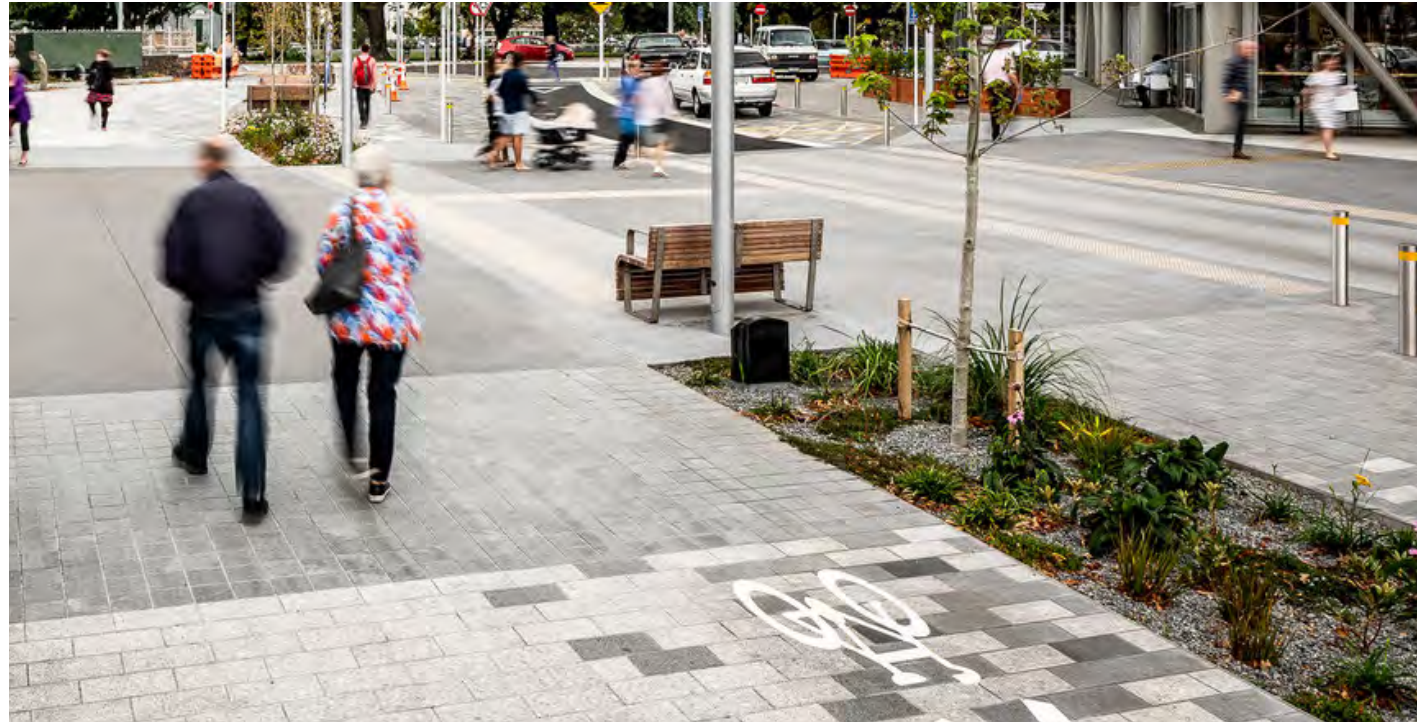
Health Precinct, Christchurch Planted rain gardens filter and clean stormwater to some extent from central city streets, delineate spaces and provide amenity.
