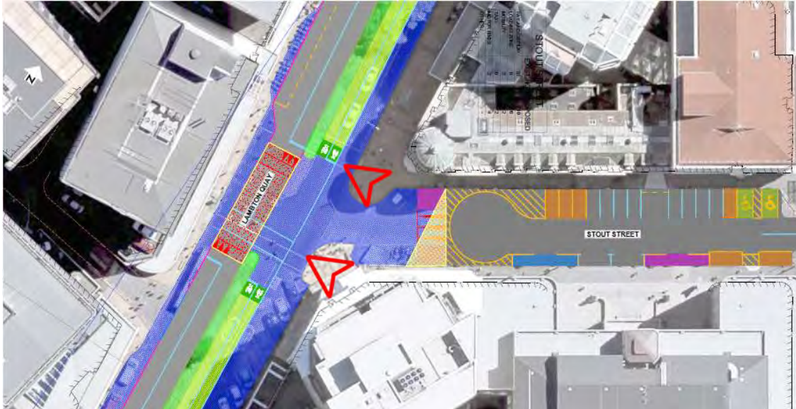
Figure 4-9: Stout Street Interface Design. Note termination of cycleway set well back from pedestrian crossing.
