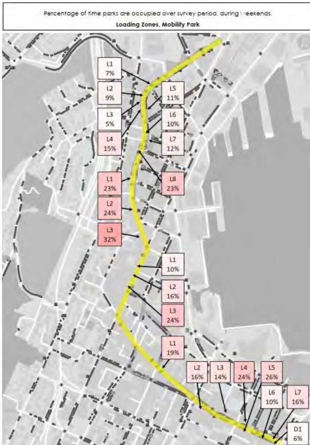
Figure 8-2: Loading zone and mobility (bottom right park only) utilization (realms for weekends) (percentage of "seats" with park occupied).
