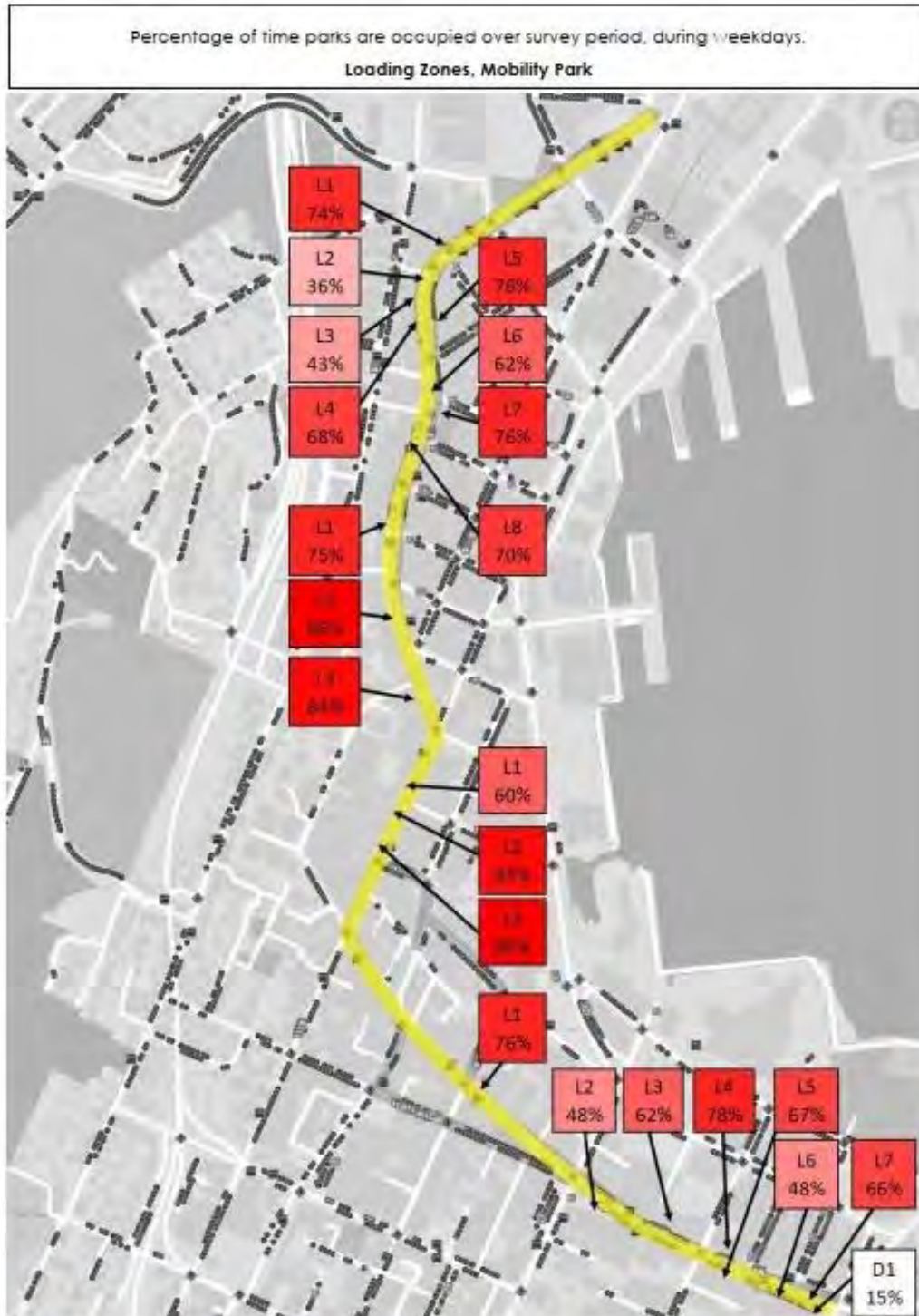
Figure 9-3: Loading zone and mobility (bottom right park only) utilization heatmap for weekdays (percentage of "beats" with park occupied)
