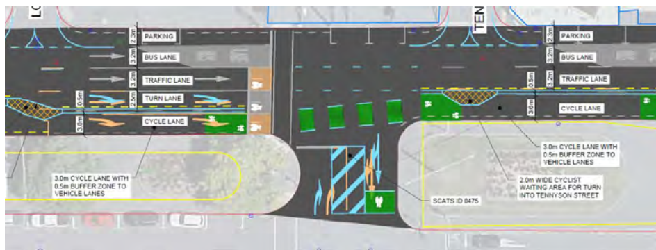
Figure 2-18: Cambridge Tce ASB at Elizabeth St intersection
