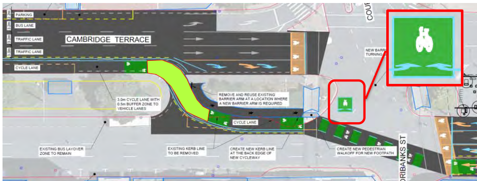
Figure 2-20: Cycle hook turn box located within intersection
