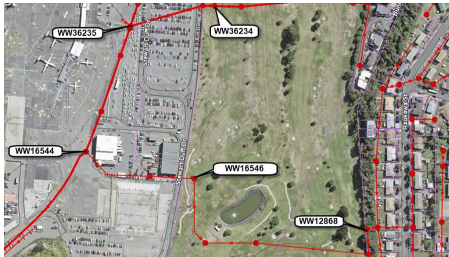
Wastewater Network Plans
