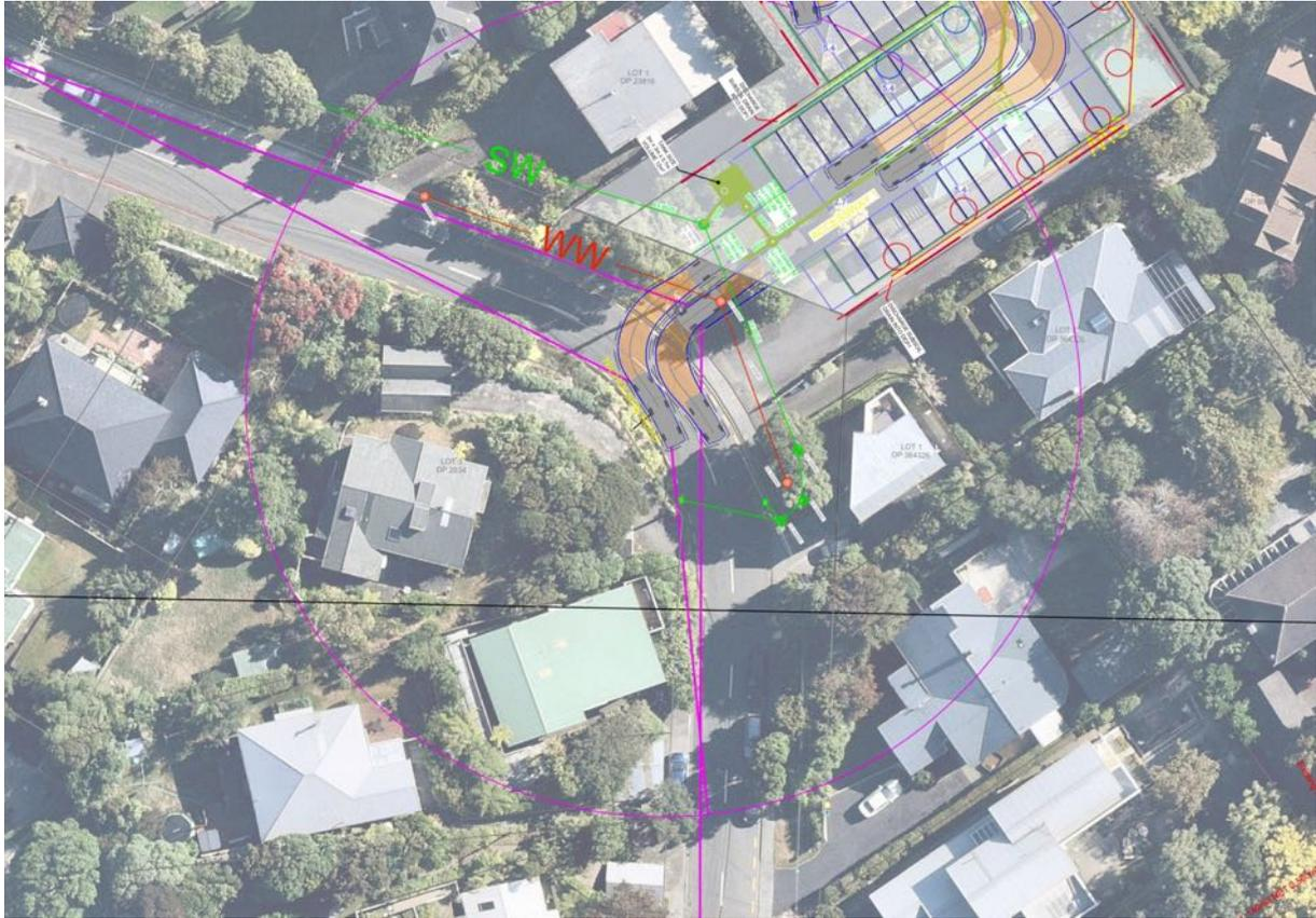
In order to achieve the required sight distance, vegetation will need to be removed on the inside of the bend within road reserve. Photograph 5 shows the required vegetation removal.
