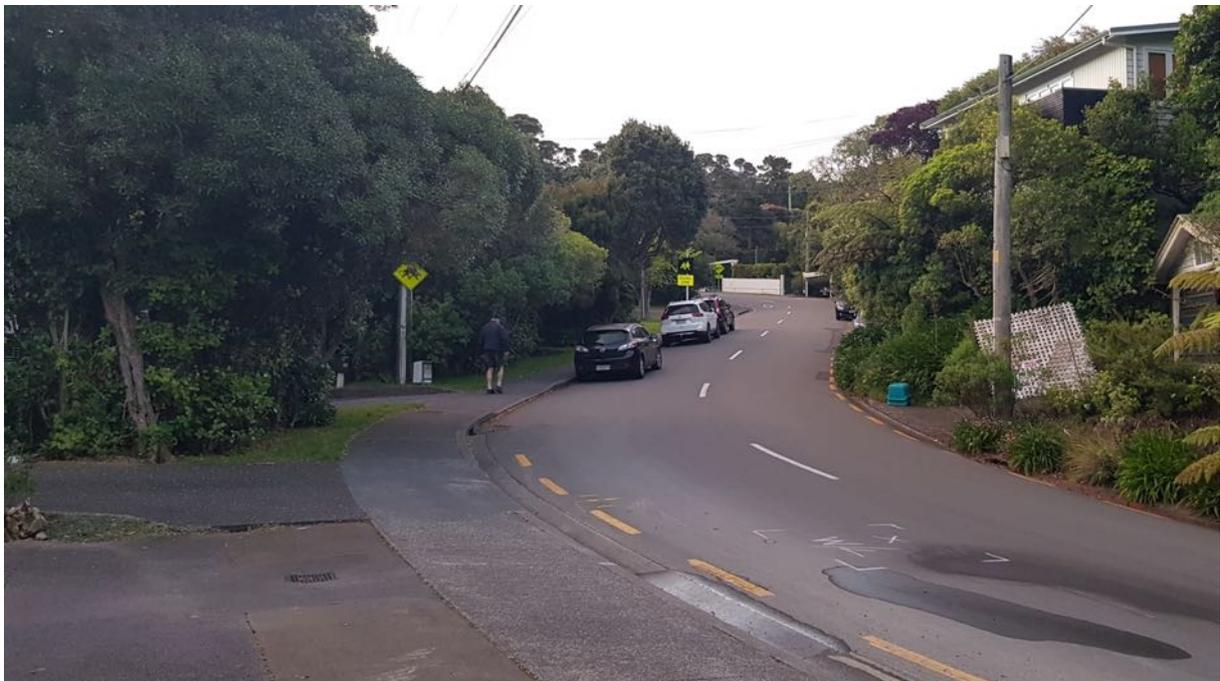
There is greater than 30 m visibility to the east and west satisfying RTS-6 requirements. Again, for completeness, we have also assessed sight distance in accordance with Austroads. The Safe Intersection Sight Distance (SISD) requirement for a 40 km/hr design speed is 73 m. This distance can be satisfied to the north and south.
