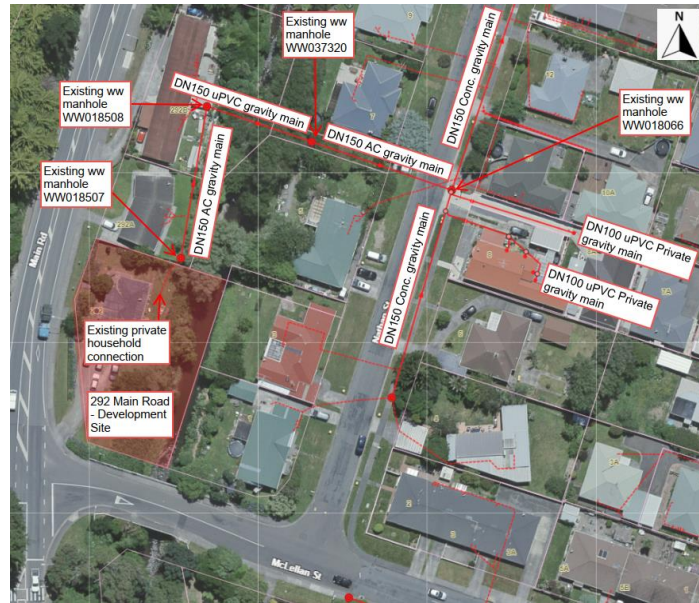
Figure 4 Existing Wastewater infrastructure assets in the vicinity in the site (Ref.: Wellington Water online GIS)
