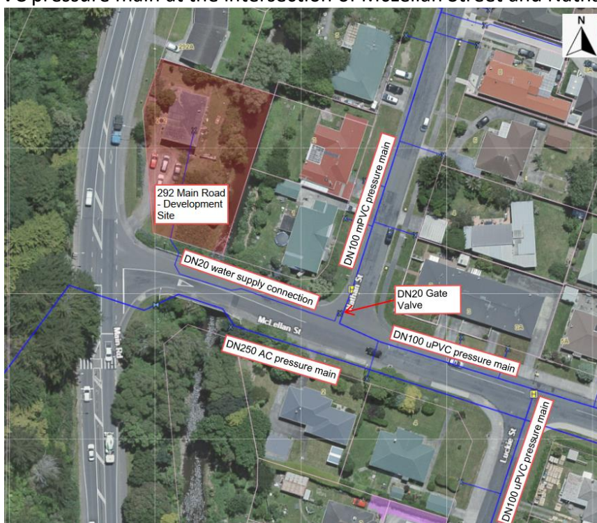
Figure 3 Existing Water Supply infrastructure in the vicinity of the site (Ref.: Wellington Water online GIS)
