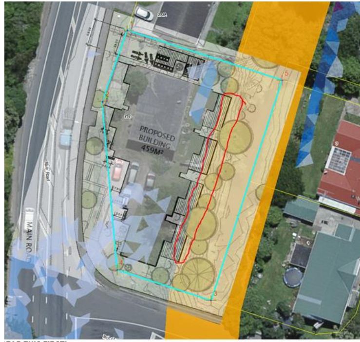
Figure 10 Modelled onsite flooding (1 in 100 year Annual Return Interval + 20% Climate Change Intensity) onsite (Ref.: ArcGIS, WCC Combined 100yearCC Flood Zones)
