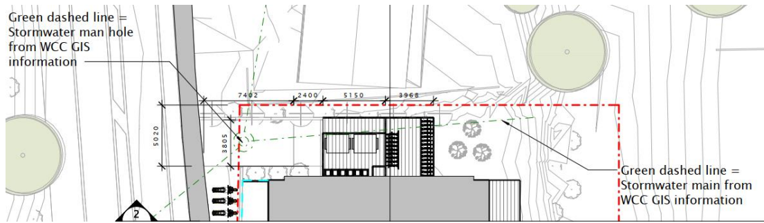
Figure 8 Applicant's Proposal to build over the existing SW main along the sites northern boundary (ref.: Archaus Drawing Set – 21026 292 Main Road Tawa – Rev 2, 28/01/2022)
