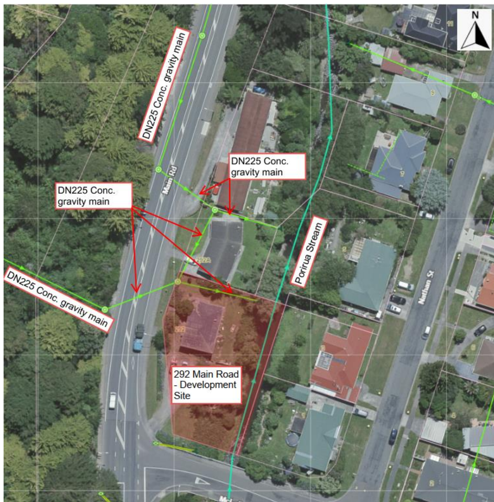
Figure 5 Existing Stormwater Infrastructure in the vicinity of the site (Ref.: Wellington Water online GIS)
