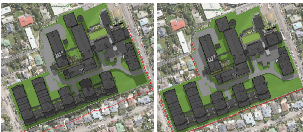
Figure 56: Afternoon sun (12noon-3:30pm) enters all the various courtyard spaces at mid-winter (image left shows 2pm, 22 June; right shows 12noon, 23 September).
