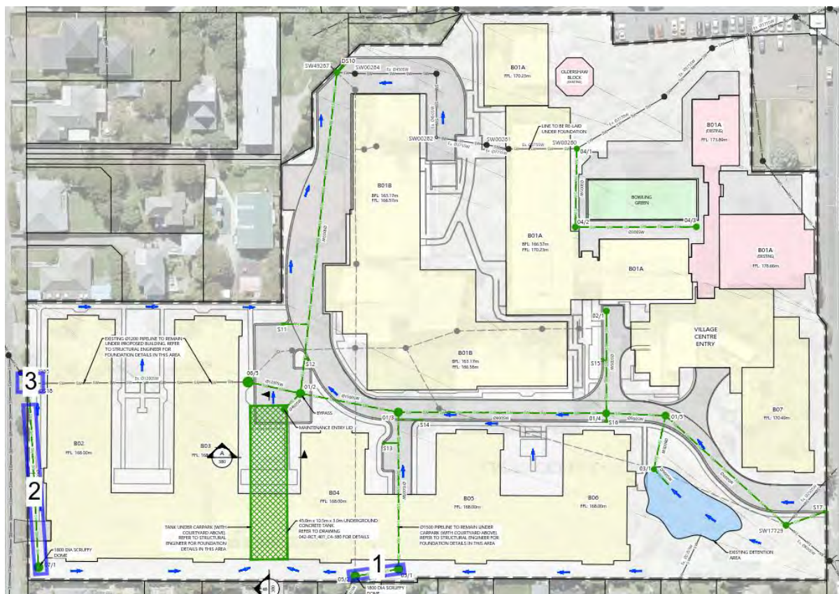
Figure 8.3: Stormwater infrastructure with potential effects on adjoining properties.
