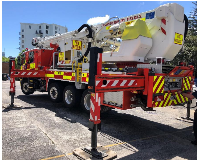
Figure 13 – Highlights the space requirements for jacking stabilisers
