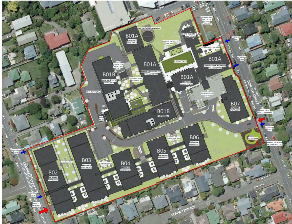
Figure 51: The Proposed Site Plan (RC04 .A0-021). B01A and B01B comprise the VC or Village Centre, Assisted Living Suites (ALS), and Care Rooms. B02-B07 contain the Independent Apartments (IA).
