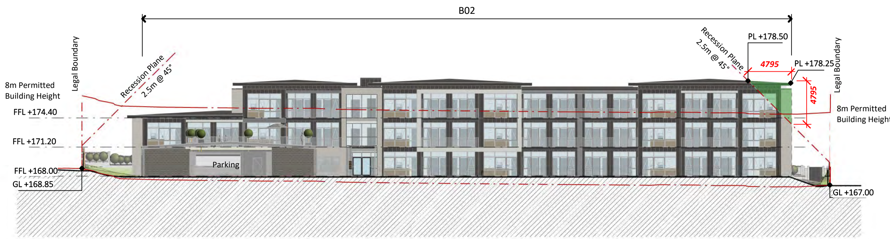
1 B02 - RECESSION PLANE SECTION A0-030 A1 sheet scale = 1 : 250 A3 sheet scale is twice scale shown above
