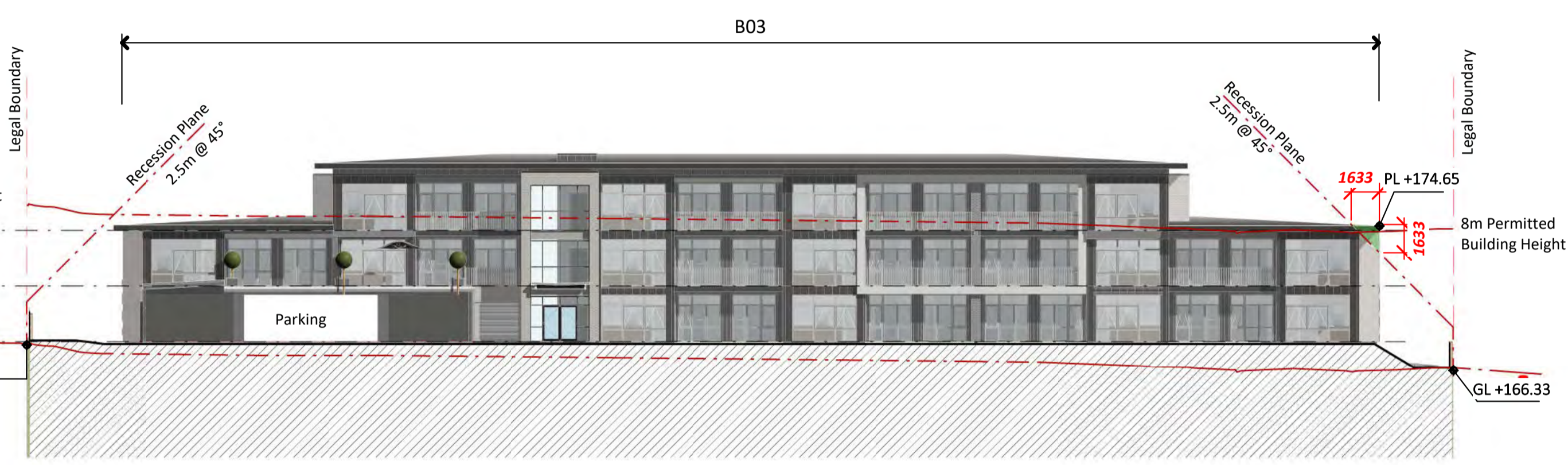
5 B03 - RECESSION PLANE SECTION A0-030 A1 sheet scale = 1 : 250 A3 sheet scale is twice scale shown above
