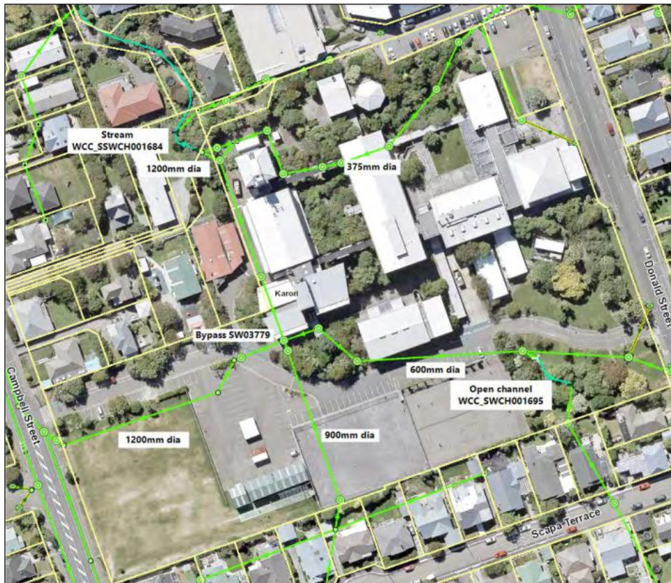
Figure 1: Existing stormwater network
