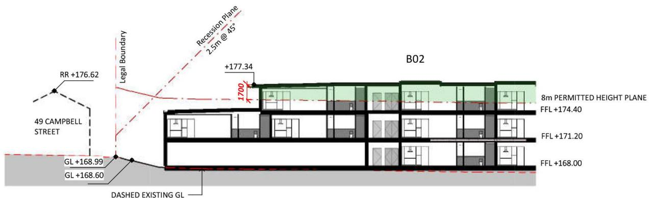
**Figure 3: Cross Section showing the relationship between Building B02 and property at 49 Campbell Street**
