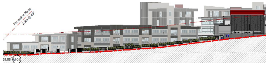
Figure 9: Allen Ward VC Hall and Building B07 front Donald Street. Building B06 is set back from the Donald Street boundary.
