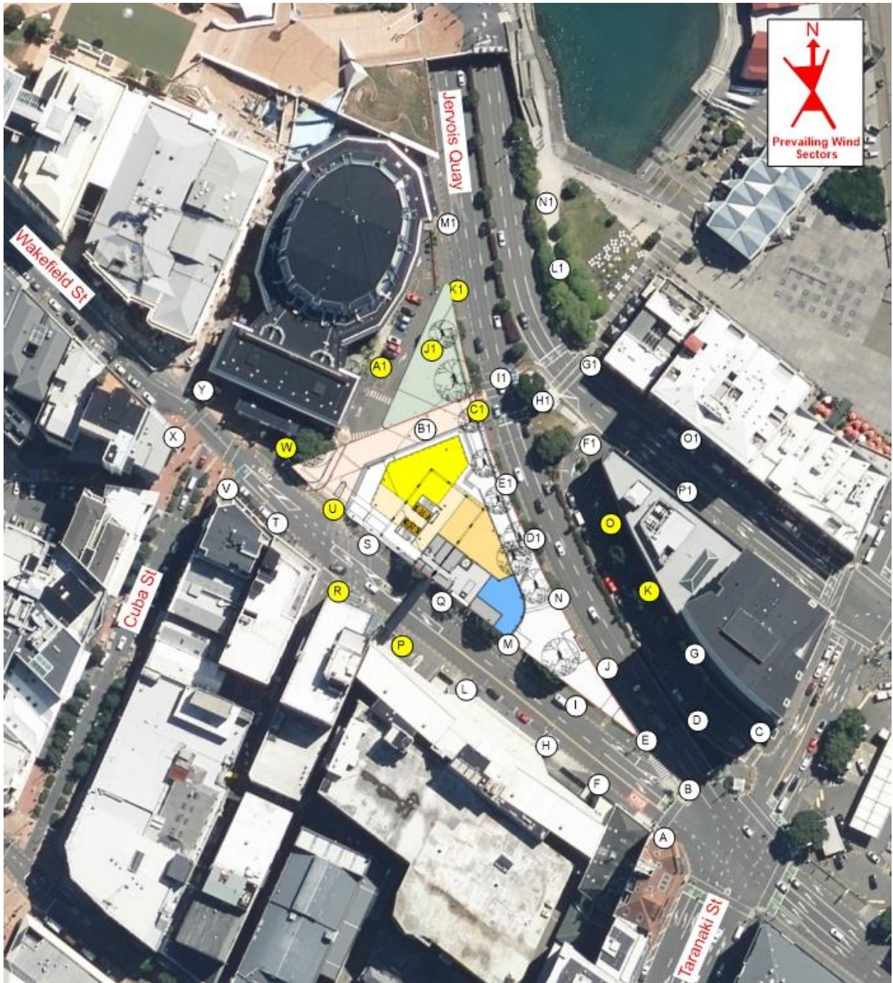
Figure 2: Wind speed measurement locations (for revised design (yellow), for original design (yellow and white))
