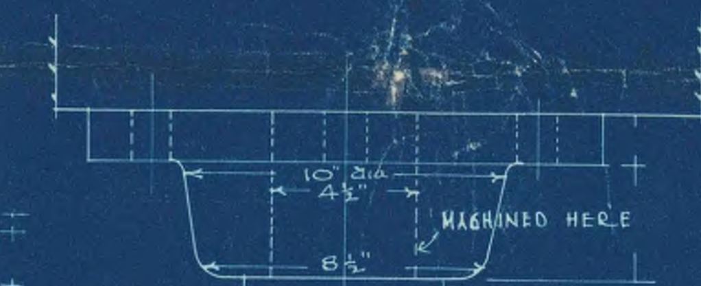
CAP OF COL. 1/4 FULL SIZE. CAP - MILD STEEL - TO BE SHRUNK ON.
