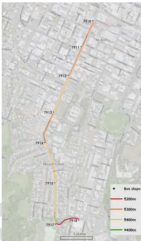
Figure 101: Bus stop locations and spacing – Inbound
