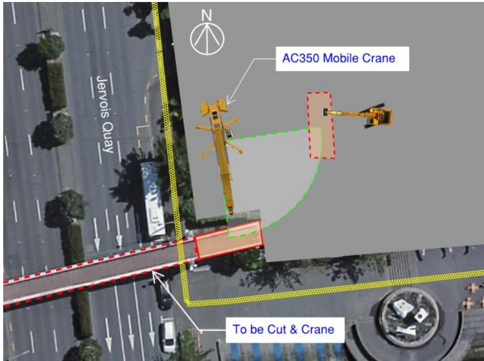
Picture 4 Section 3 Bridge Cut & Crane Step 1
