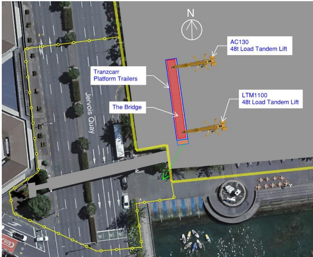
Picture 6 Section 3 Bridge Cut & Crane Option 1 – B
