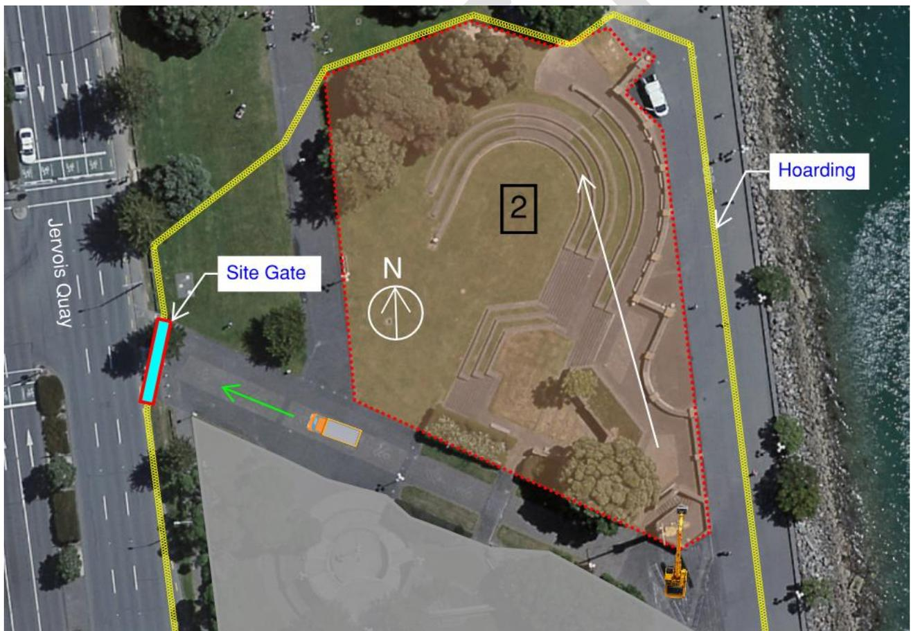
Picture 3 Section 2 Demolition Plan
