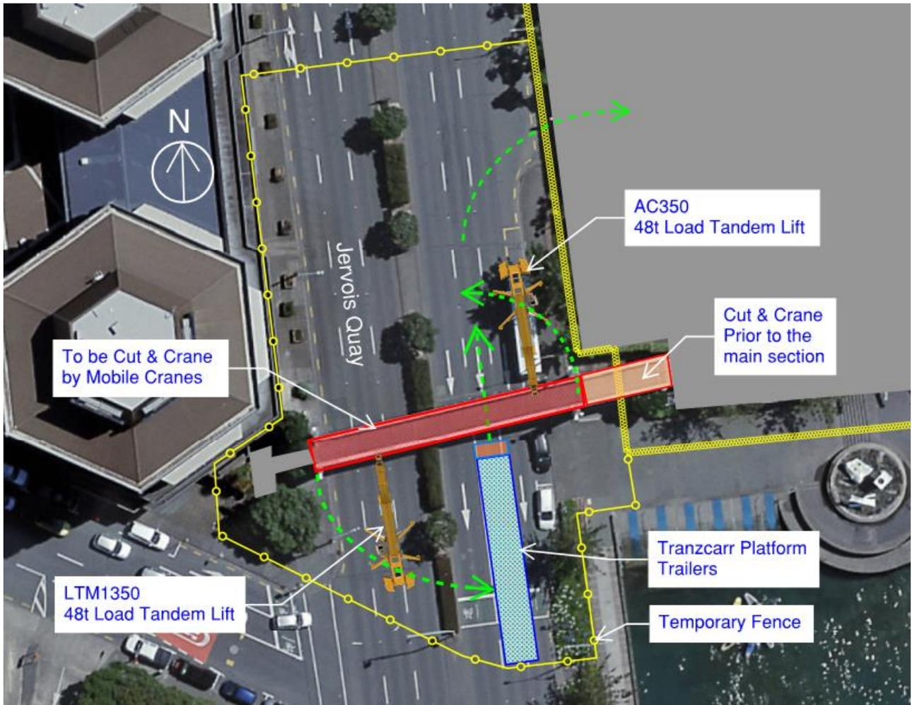
Picture 5 Section 3 Bridge Cut & Crane Option 1 – A
